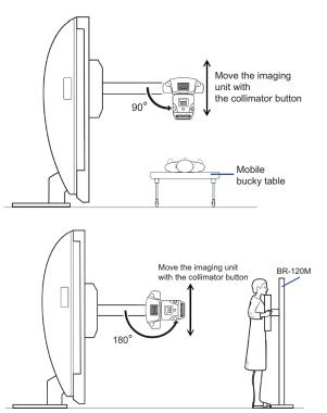
Fix the X ray tube with grip bar at 0°, 90° or 180°.
