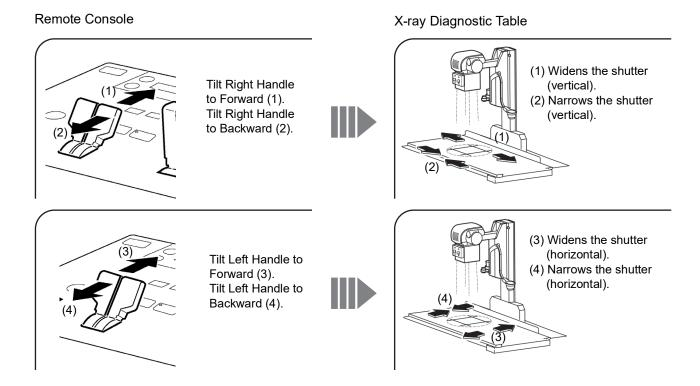
Adjusting Manually by Collimator Knobs (when using FPD portable radiography)
