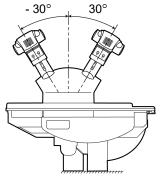
Fig 1.3 Tilting X-ray Tube
